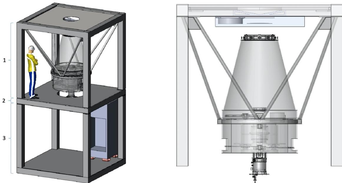
Figure 9. The ComCam IMF is split into three sections, shown on the left. A GMT-standard electronics cabinet is shown on the lower level. The upper section, which includes the ComCam mounting ring and support struts, is shown on the right with the instrument installed. A protective hatch assembly is attached inside the top of the IMF.
