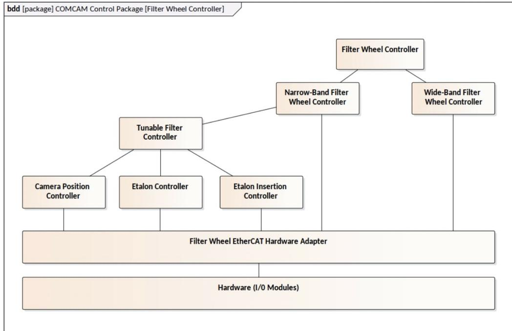
Figure 16. Example software component package block diagram: filter controller.
