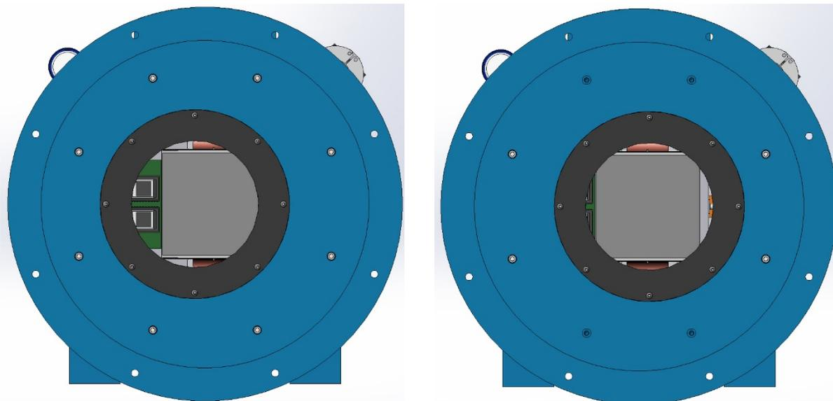
Figure 14. CCD camera face plate in two orientations, one centered on the science CCD (right) and one that accommodates the flexure/focus CCDs (left).
