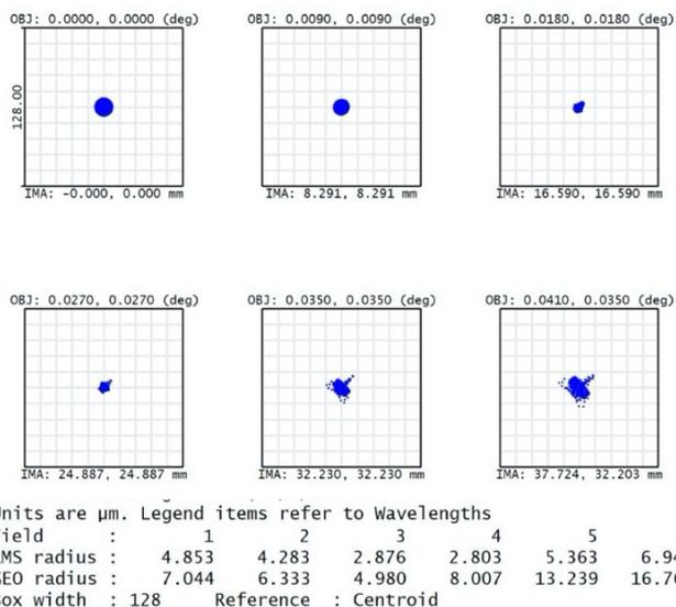
Figure 5. Example spot diagram for  $\lambda 550$  nm in a 0.5 arcsec box. Field positions are shown in Figure 2.
