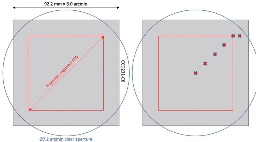
Figure 2. Optimization and clear aperture relative to both the CCD and the required FOV. The right panel shows the field positions corresponding to the image quality evaluation numbers given in Table 2.
