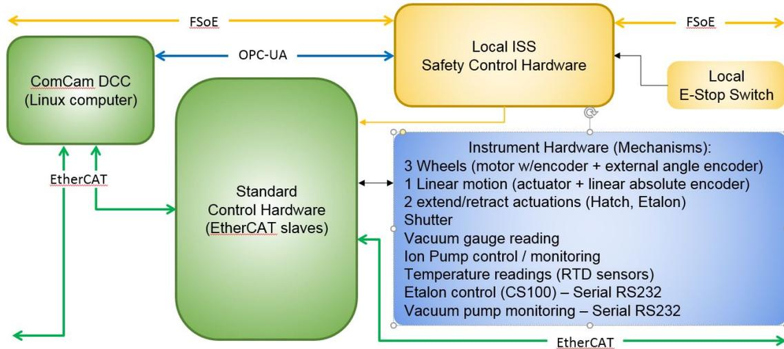
Figure 15. Controls communication flow diagram. Abbreviations: Device Control Computer (DCC), Interlock and Safety System (ISS), Safety over EtherCAT (FSoE), Open Platform Communications - Unified Architecture (OPC-UA)
