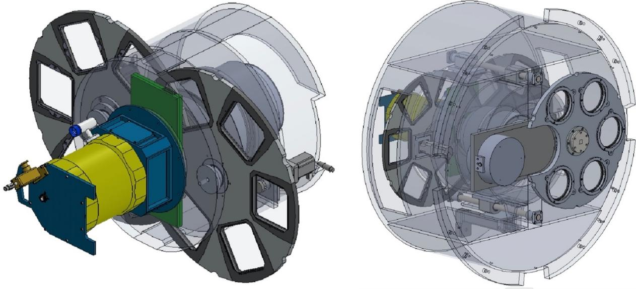
Figure 11. Filter deployment. Shown on the left, two wideband filter wheels, each with six positions, mount just in front of the shutter and detector packages. On the right, from a different angle and at a different scale, the narrowband filter wheel and a block concept for an etalon insertion mechanism are shown.
