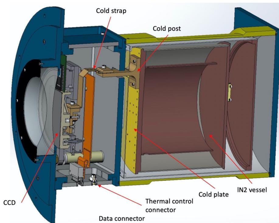
Figure 13. CCD camera in cross-section.
