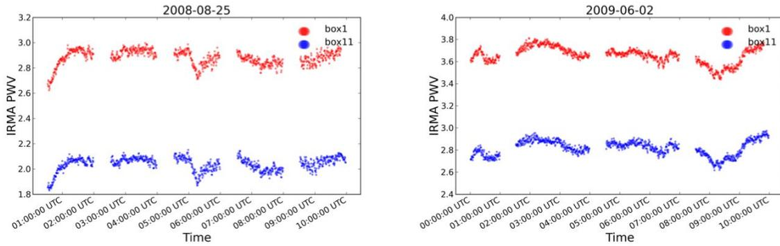
Figure 3. Two examples of the variation of pwv over the course of a night as measured by both IRMA units. These have not been calibrated via the MIKE calibration to show the offset in absolute calibration. The two instruments clearly see the same temporal variation.
