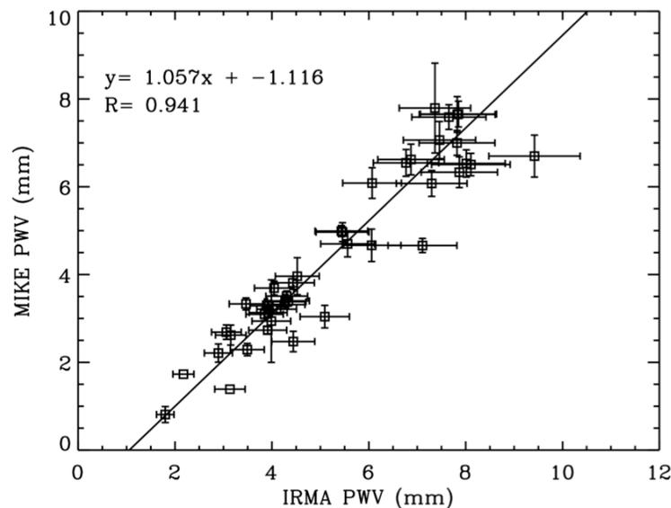
Figure 6. The correlation between MIKE PWV and IRMA PWV. Linear fit and correlation coefficients displayed in upper left. MIKE error bars are standard deviations for the means of the 5 different optical pwv lines measured. IRMA error bars are set to 10% in the absence of a true uncertainty calculation based on a reduced chi-squared near one in the above fit. The uncertainties on the coefficients are 0.050 and 0.282.
