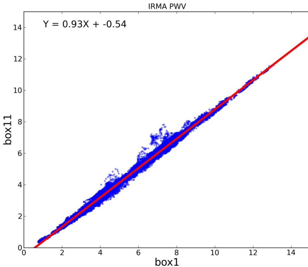
Figure 4. Correlation between the PWV as measured by the two different IRMA units. The relative rms error between these data sets is 5% indicating reasonable precision between the units.
