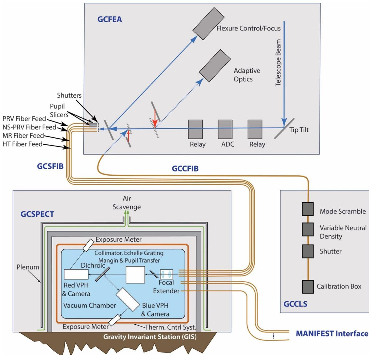
Figure 1:G-CLEF system diagram showing the major subsystems.
