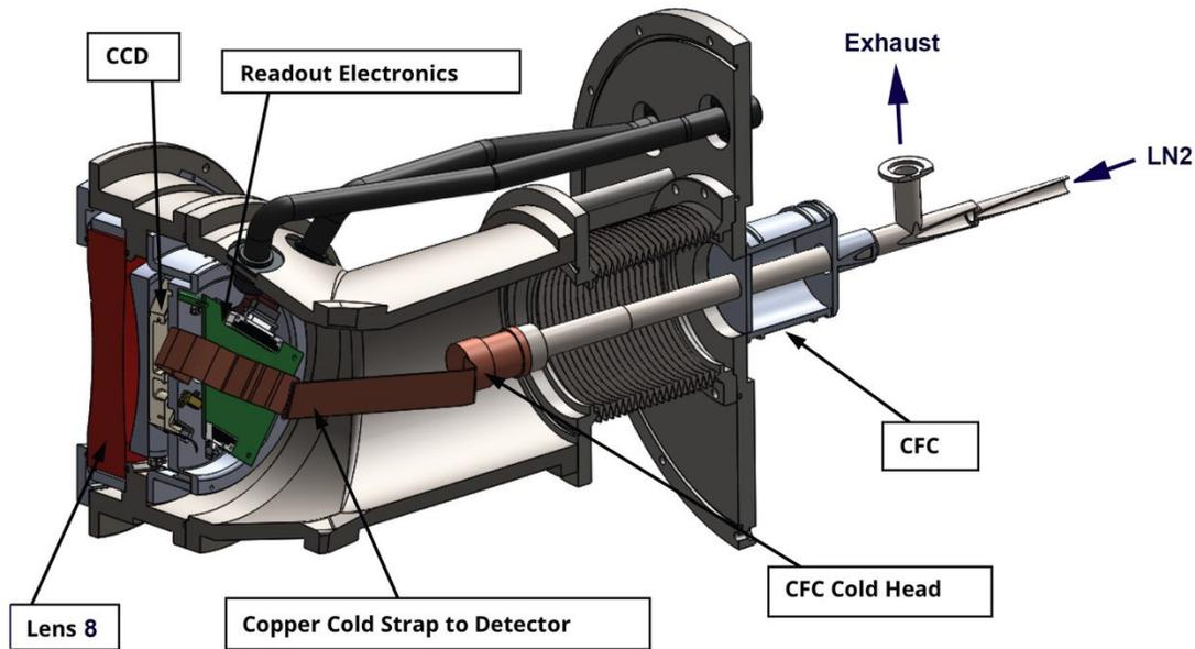
Figure 12: Red camera CCD cryostat in section.
