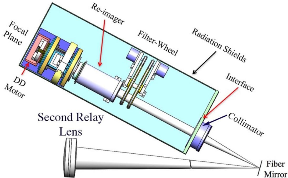
Figure 18: The G-CLEF FCC mechanical design.
