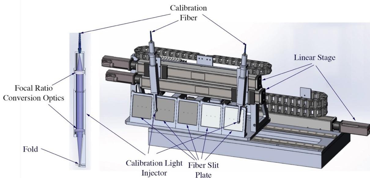
Figure 6: Physical implementation of the fiber feed/selector. A section view of a calibration light injector is shown on the left panel.
