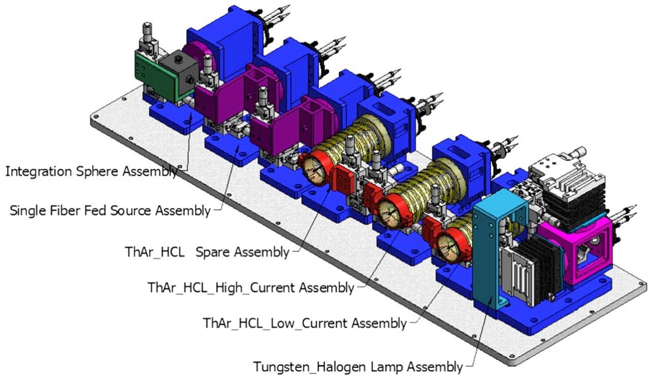
Figure 19: Calibration lamp light sources at PDR.
