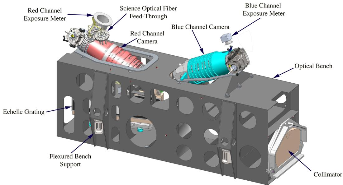
Figure 9. Major elements of the spectrograph mechanical design.
