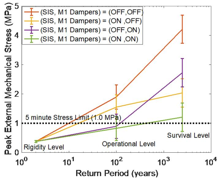
Figure 3: Effect of the GMT Seismic Isolation System (SIS) and M1 support actuator damping on mirror stress<sup>4</sup>
