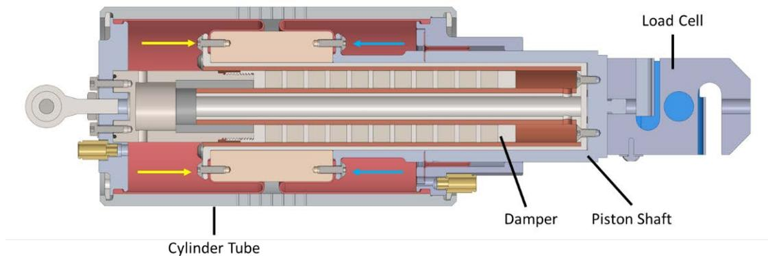
**Figure 9: Support Actuators Air Cylinder Cross Section with Eddy Current Style Damper**
