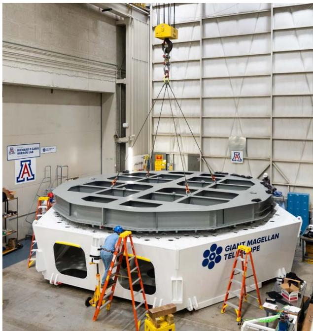
**Test Cell Integrated with Mirror Simulator**
