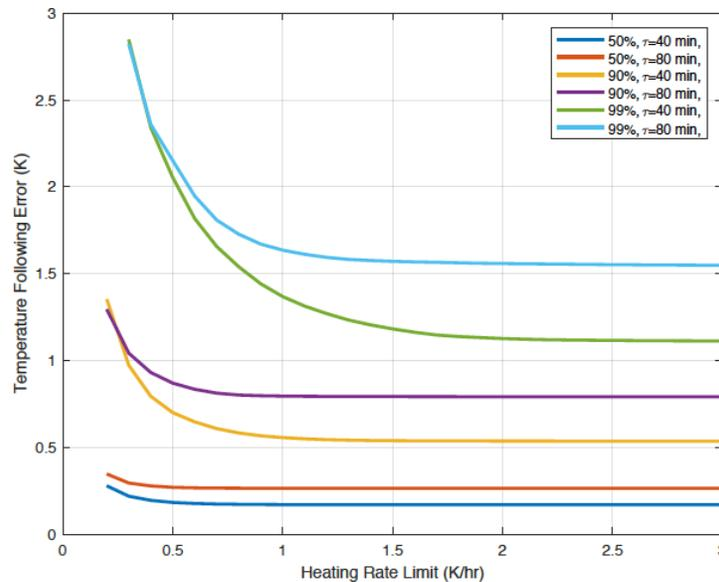
Figure 4: Median and 90<sup>th</sup> percentile temperature following error as a function of thermal time constant and heating/cooling rate limit<sup>5</sup>
