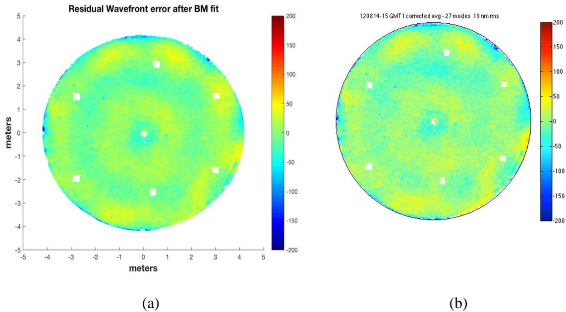
**Figure 5: Mirror polishing error after active optics correction. Surface map is in nm. The first 27 bending modes of the mirror are corrected. (a) Simulation results from GMTO. (b) Simulation results from the University of Arizona Richard F. Caris Mirror Lab.**
