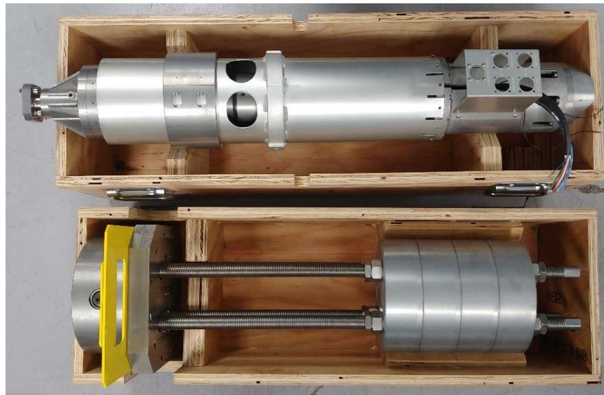
**Figure 10: Hardpoint Actuator and Counter-balance Weight Assemblies**
