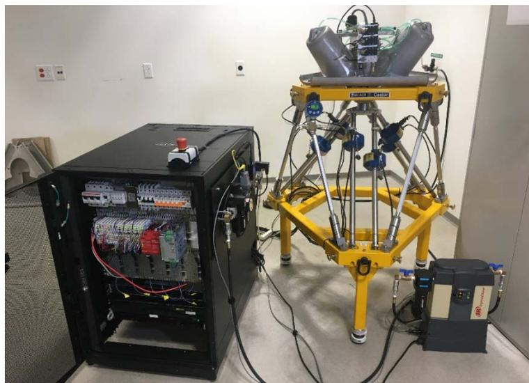
**Figure 8: M1 Actuator Calibration Stand with Motion Stage**
