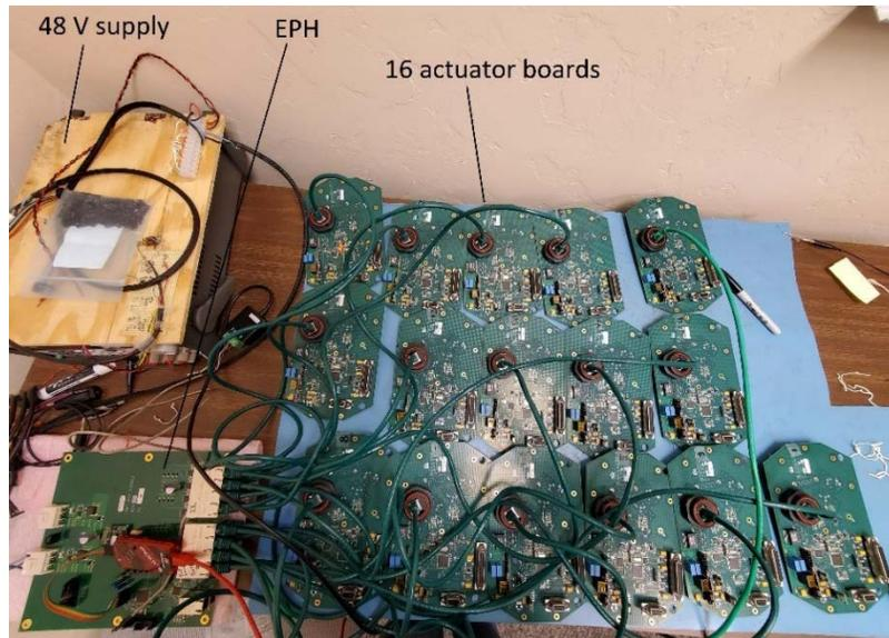
**Figure 12: EtherCAT and Power Hub Board (EPH) with 16 Support Actuator Boards**
