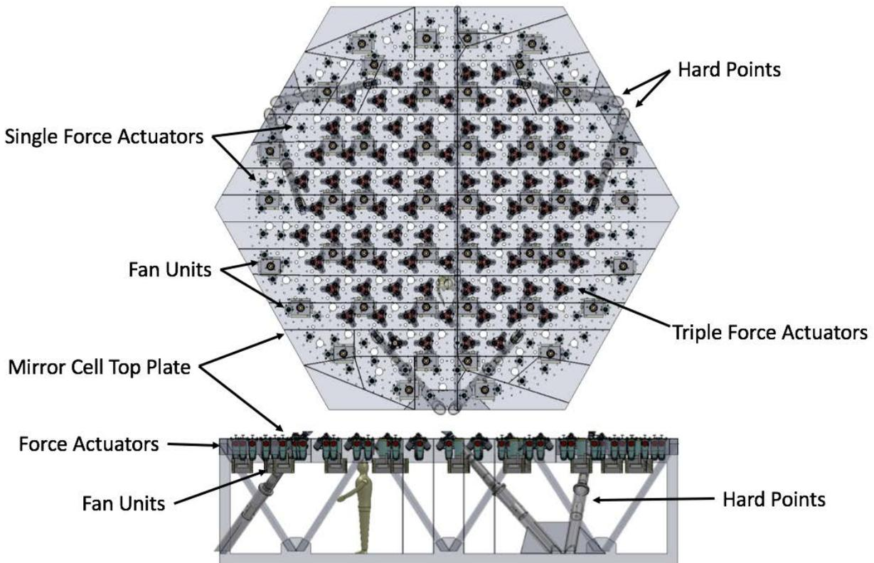
Figure 1: M1 Subsystem Layout within an Off-Axis Mirror Cell
