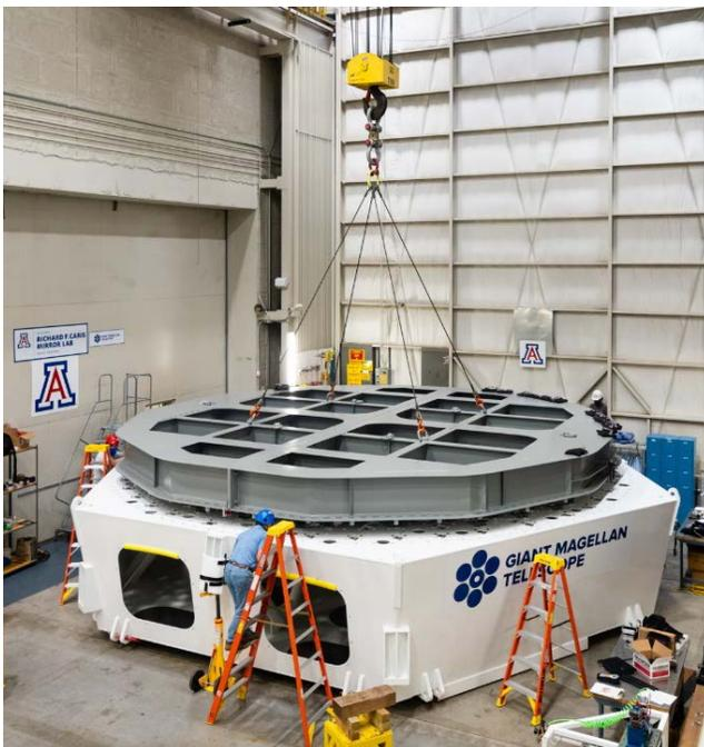
**Test Cell Integrated with Mirror Simulator**
