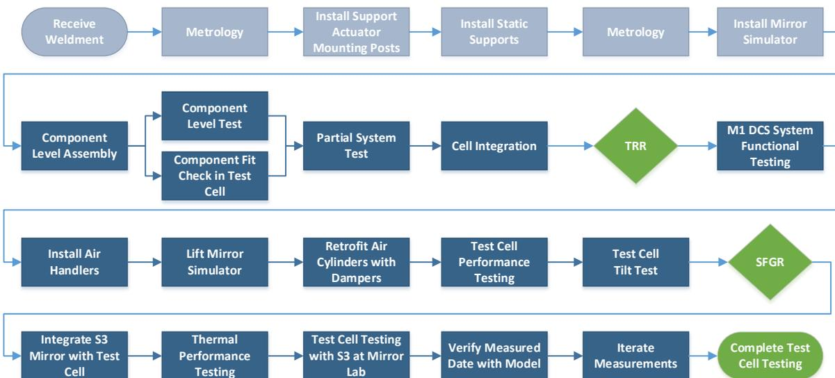
Figure 14: Test Cell Integration and Test Flow Diagram (grey signifies completed)
