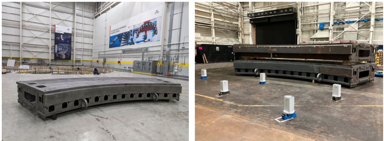
Figure 14. Sections of the Azimuth Track at IMT in Rockford, IL prior to being shipped to Huntsville, AL for rough machining by Teledyne. The section on the left has completed grit blasting while the two sections on the right are awaiting grit blasting. (Photos courtesy of Ingersoll Machine Tools)
