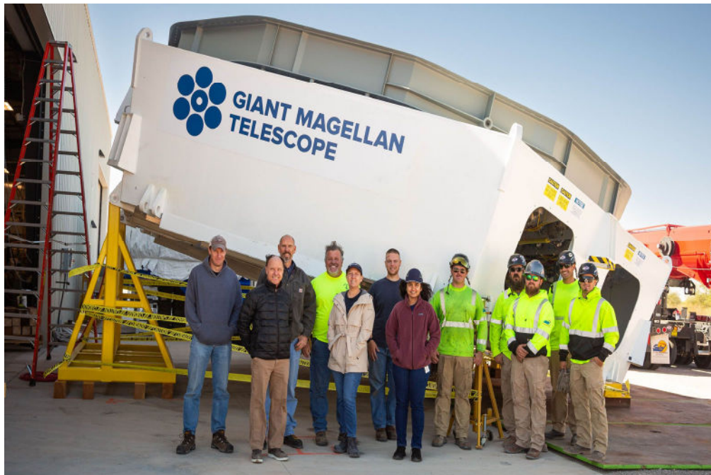
Figure 4. The GMT M1 Test Cell weldment (white) with a full scale mirror simulator (gray) tilted at 14 degrees which is the angle an off-axis mirror segment will be when the telescope is at its zenith-pointing position. The Test Cell is now fully functional with its mechanical support system and under full software control (an image of the user interface for this control system is shown below in Figure 23).
