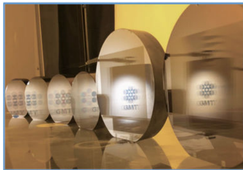
Figure 19. Immersion gratings for GMTNIRS. (Photo courtesy of Ben Kidder)
