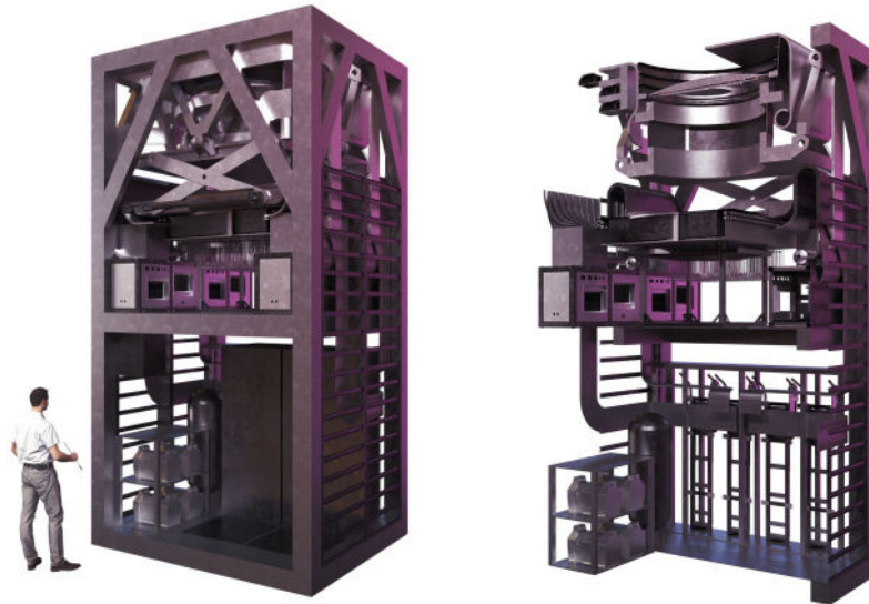
Figure 21. Exterior view of the MANIFEST fiber positioning system in its interface mounting frame (right) and cutaway section view (right).
