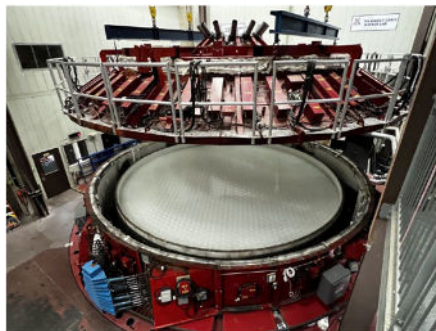
Figure 3. S7 initial production activities: the loading of the glass into the mold (left), the opening of the hearth after the mirror is cast (center), and post-casting cleanout of the cast mirror.
